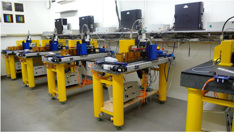
Fig. 4. The emulsion scanning station of the Bern OPERA group equipped with 5 automatic microscopes.
