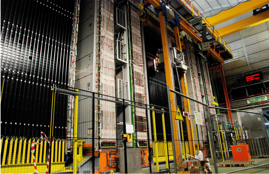
Fig. 2. The OPERA detector in the LNGS underground Hall C.
