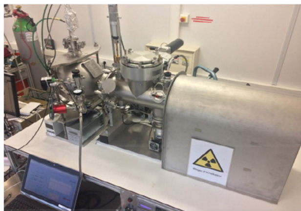
Fig. 2 A picture of the experiment with Comimac on the right and the SPC on the left
