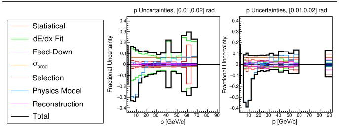
FIG. 12. Systematic uncertainty breakdown for 2016 and 2017 p analyses. One representative angular bin is shown.
