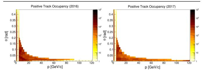
FIG. 2. Binning scheme and track occupancy comparison for positive tracks between 2016 dataset (left) and 2017 dataset (right) for the proton analysis. Note the significantly increased phase space occupancy in the forward region for the 2017 analysis. This is the result of adding the FTPCs to the NA61/SHINE detector. The empty region at low momenta corresponds to the omitted Bethe-Bloch crossing region for protons and pions.
