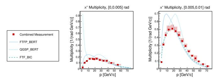
FIG. 17. Combined multiplicity measurements for  $\pi^+$  analysis. Error bars denote statistical uncertainty, and total systematic uncertainty is shown as a shaded band. Results are compared to three Monte Carlo models. Two representative angular bins are shown.
