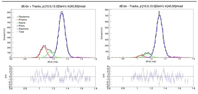
FIG. 5. Example dE/dx distribution fit for one kinematic bin showing positively (left) and negatively (right) charged track distributions. This kinematic bin shows an abundance of pions in both the positively and negatively charged track distributions, a significant fraction of protons, and a lack of antiprotons. This is characteristic of the 120 GeV/c proton-carbon reaction.
