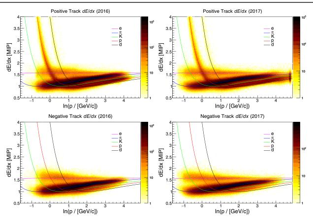
FIG. 4. Two-dimensional distributions of charged track dE/dx vs.  $\ln(p)$  for the 2016 and 2017 datasets after applying track quality cuts. The lines represent Bethe–Bloch predictions for various particle species. Increased acceptance in the 2017 dataset is visible in the extension of the distribution to lower total momenta (due to a lower magnetic field setting) and a prominent peak in positively charged track dE/dx at the beam momentum  $(\ln(p/[\text{GeV}/c]) = 4.78)$ .
