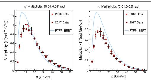
FIG. 8. Example  $\pi^{\pm}$  multiplicity measurements comparing the 2016 and 2017 analysis results. Uncertainties reflect total uncertainty (statistical and systematic) for the independent analyses.
