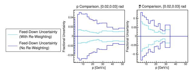
FIG. 7. Comparison of uncertainties associated with feed-down correction with and without the inclusion of neutral-hadron multiplicity measurements as constraints [15]. Uncertainties are reduced from up to 5% to less than 2% for p (left) and from more than 10% to around 6% for  $\bar{p}$  (right). Only one representative angular bin is shown.
