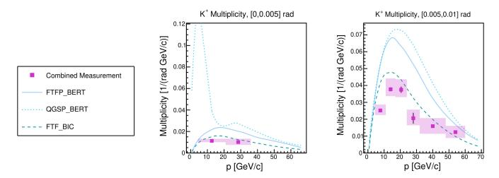
FIG. 21. Combined multiplicity measurements for  $K^+$  analysis. Error bars denote statistical uncertainty, and total systematic uncertainty is shown as a shaded band. Results are compared to three Monte Carlo models. Two representative angular bins are shown.
