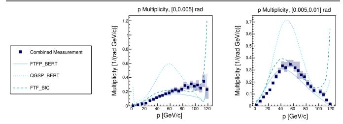
FIG. 19. Combined multiplicity measurements for p analysis. Error bars denote statistical uncertainty, and total systematic uncertainty is shown as a shaded band. Results are compared to three Monte Carlo models. Two representative angular bins are shown.
