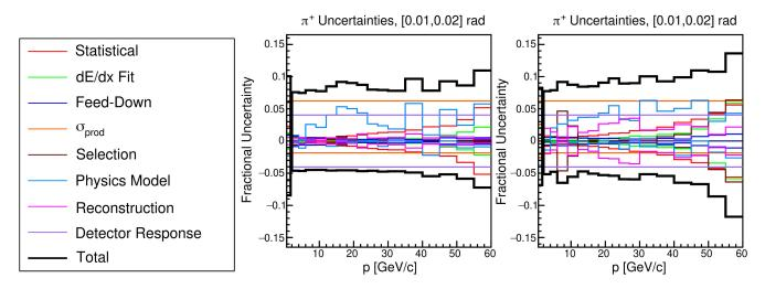
FIG. 11. Systematic uncertainty breakdown for 2016 and 2017  $\pi^+$  analyses. One representative angular bin is shown.
