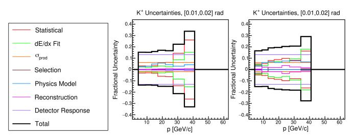
FIG. 13. Systematic uncertainty breakdown for 2016 and 2017  $K^+$  analyses. One representative angular bin is shown.
