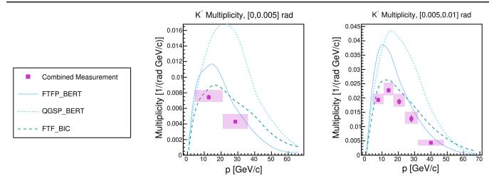
FIG. 22. Combined multiplicity measurements for  $K^-$  analysis. Error bars denote statistical uncertainty, and total systematic uncertainty is shown as a shaded band. Results are compared to three Monte Carlo models. Two representative angular bins are shown.
