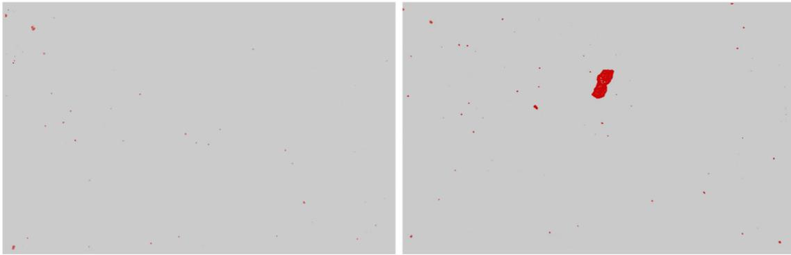
**Fig. 2** Optical images of clean (left) and dirty (right) witness coupons, post optical processing. The feature common to them are dust from the optics, and serves as a calibration check
