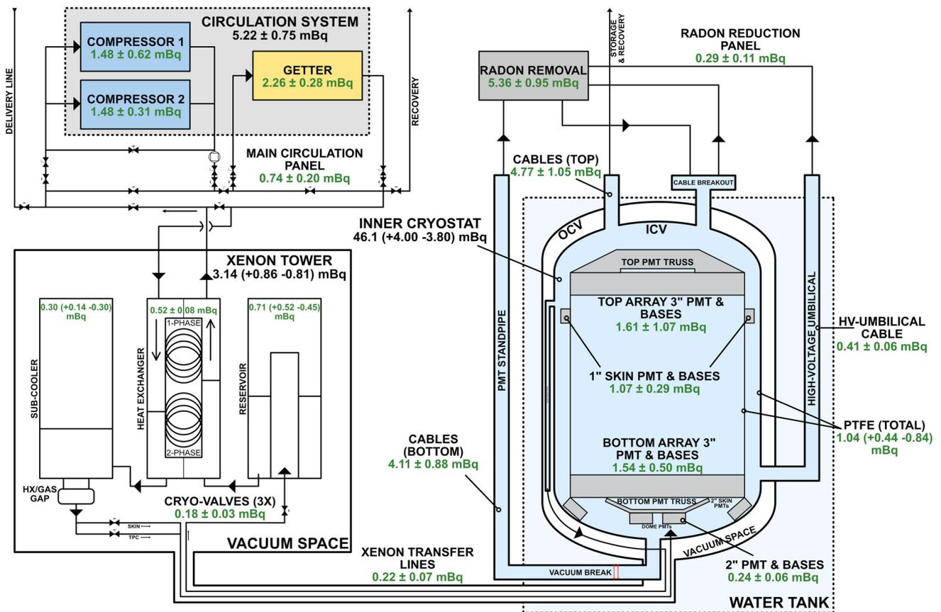
**Fig. 7** Approximate schematic of LZ highlighting key sub-systems and xenon circulation paths in and out of the ICV. The diagram condenses some of the key radon emanation measurements that will contribute to the overall radon budget of LZ. The results presented in green text are directly from measurements and those in black show summed
