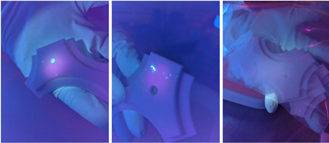
**Fig. 4** Pictures of some PTFE components (used on the PMT arrays) under UV light before (left and center) and after (right) cleaning with IPA saturated non-shedding mono-filament wipes. Fluorescent specks are dust particulates which are removed after cleaning the pieces in an IPA bath as seen in the right picture
