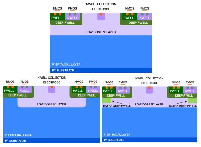
Fig. 2 Cross sections of the process modifications of the Tower Semiconductor 180 nm CMOS imaging technology. Top image shows the standard modified process (STD) where an  $n^-$  layer is introduced on top of the p-type substrate. Bottom left image shows the process modifi-
