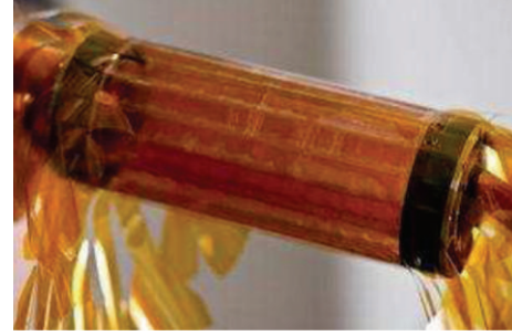
FIGURE 21: Mechanical prototype of the Mu3e inner pixel detector [107].
