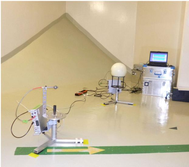
**Fig. 10** Experimental arrangement used for the DS-3 measurement (reactor ON). The bare detector in the foreground was used as a monitor of the thermal neutron fluence rate. The Bonner sphere in the back was placed in the central CONUS position. Other Bonner spheres were placed on this position one after another
