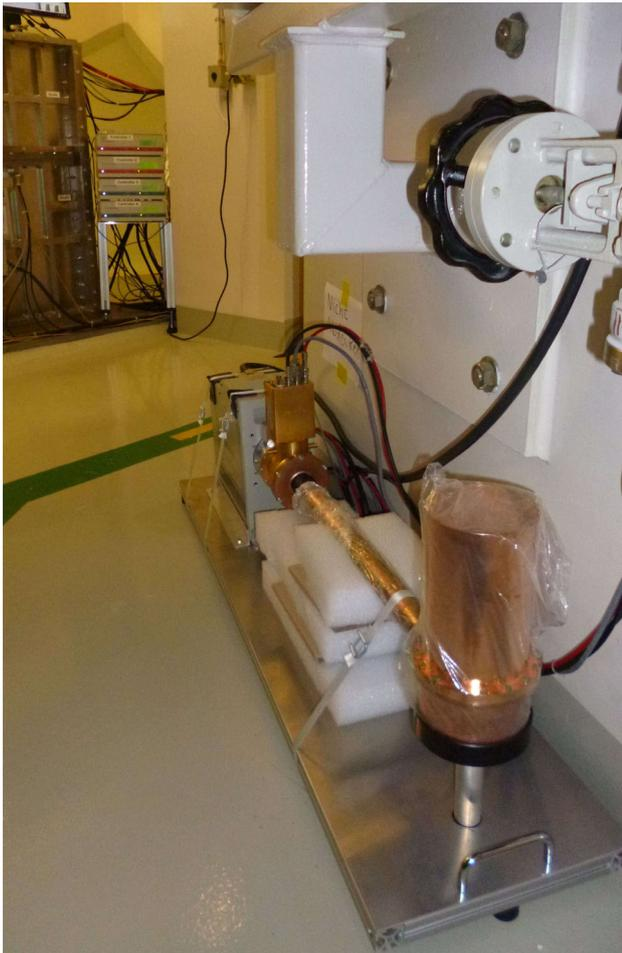
**Fig. 20** CONRAD detector at room A408 of KBR. The Cu cryostat with the HPGe diode has been placed near the closest wall to the reactor core
