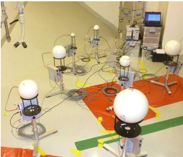
**Fig. 11** Experimental arrangement used for the DS-1 (reactor ON) and DS-2 measurement (reactor OFF). The Bonner spheres were distributed around the central position of the future CONUS setup. The bare detector is located at the central position
