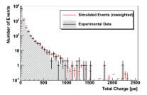
Fig. 12 Simulated events (red) re-weighted to the unfolding result (Fig. 13) compared to real data (black) for the total charge collected in an event  $Q_{\rm tot}$
