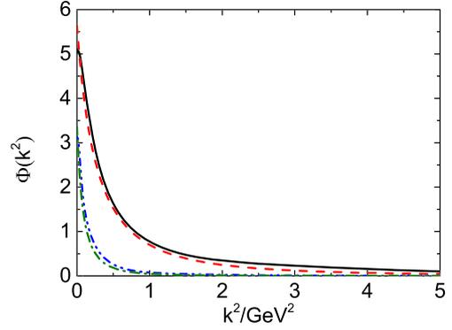
Fig. 2. The computed  $\eta_c$  meson's wave function (solid curve) and  $\pi$  meson's (dot-dashed curve) compared with the input ones (dashed curve) and (dot-dot-dashed curve), respectively.
